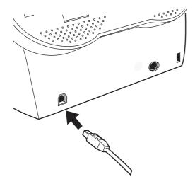
2. Connect the other end of the USB interface cable to the PC.
