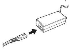
2) Connect the AC adapter connector to the scanner's DC inlet.
